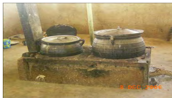
Fig. 5: Double-pot improved stove by SERC, Sokoto
