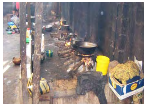
Fig. 2: Inefficient fuelwood stoves
