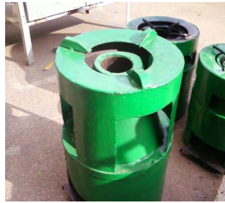
Fig. 11: Metal Efficient Stove by NCERD, Nsukka
