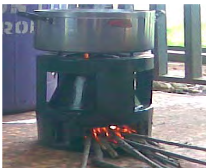
Fig. 10: Metal Efficient Stove by NCERD, Nsukka
