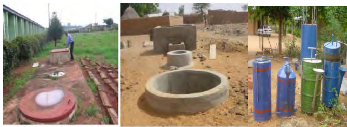
Fig. 12, 13 & 14: Biogas Digester Pilot Plant and portable floating type developed by NCERD, Nsukka and SERC Sokoto respectively
